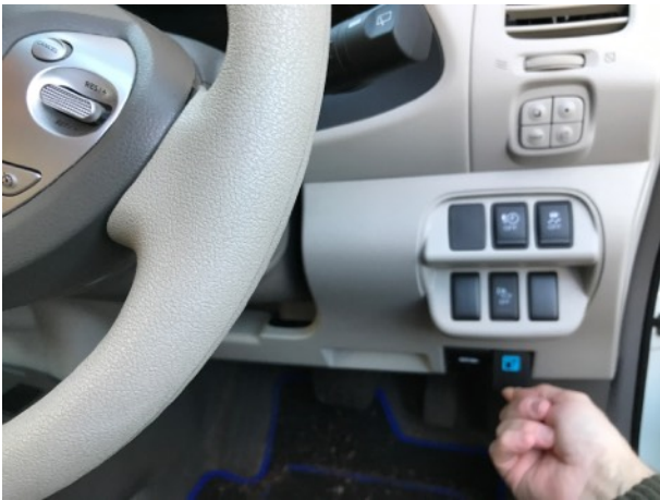
Pull lever to open flap (Nissan)
