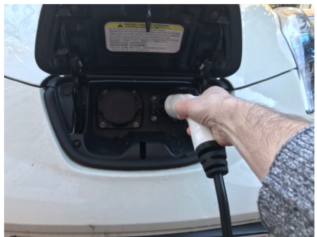
Plug in charging lead (Nissan)
